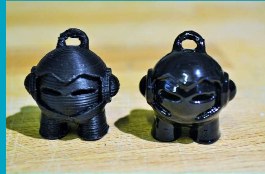
Figure 5: Example of acetone vapour smoothed part
