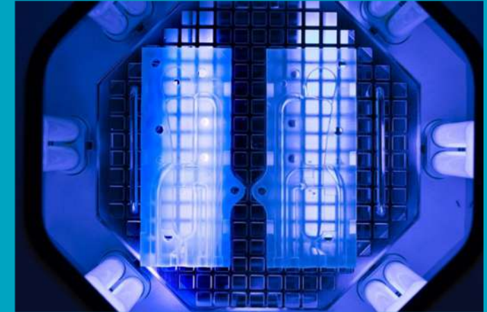
Figure 9: Post-curing parts under UV light. [5]
