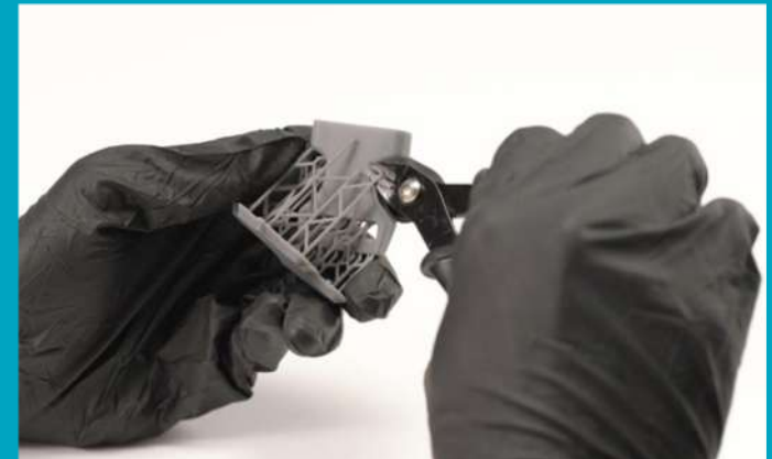
Figure 10: Removing supports with flush cutters. [5]
