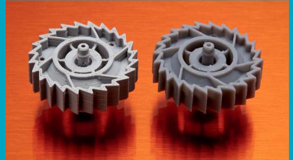
Figure 9: FDM (left) vs SLA (right). [1]
